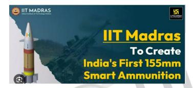
✓ The objective is to increase the accuracy of 155 mm shell within a Circular Error Probable (CEP) of 10 m. At present, ammunitions developed in India has a CEP of 500 m. Another goal is to increase the lethality at the terminal impact point.
