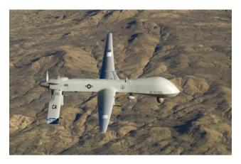
✓ The fighter-sized Predators are armed with air-to-ground missiles and smart bombs as well as capable of flying for 35 hours at a stretch.
