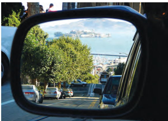
Used as rear view mirrors in automobiles since it has a wide field of view.
